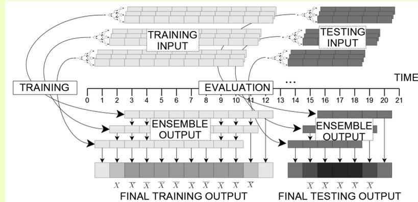
FIGURE II: Prediction System Scheme II
