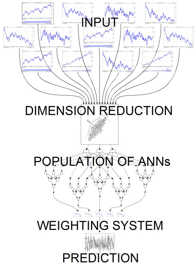
FIGURE I: Prediction System Scheme I
