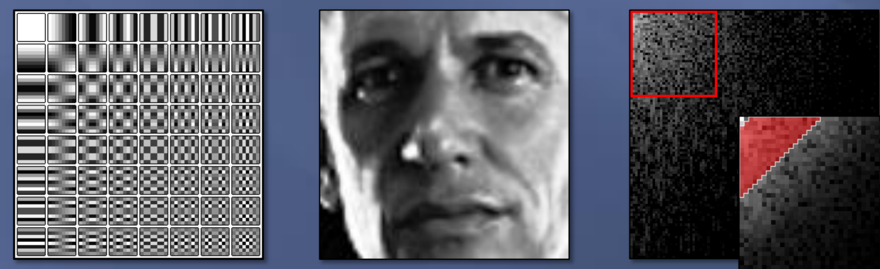
Example 8x8 DCT basis functions, and DCT visualisation for a face image
